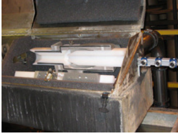
Sonic installed its drying equipment at the end of extrusion line cooling tank in its Statesville plant. Space constraints required the air knives to fit in a clam-shell enclosure (shown open).
