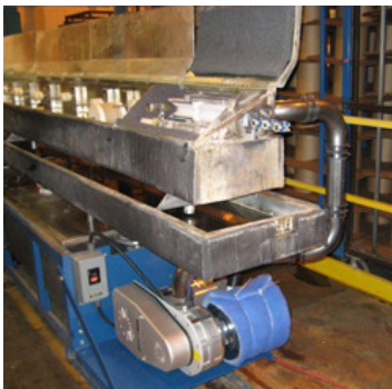
Sonic installed its drying equipment at the end of extrusion line cooling tank in its Statesville plant. Space constraints required the air knives to fit in a clam-shell enclosure (shown open).
