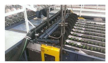
The Sonic equipment has been in operation since March 2013. "It needed only slight adjustments. We had to align the air knives with the track and figure out how much air pressure to use. A Variable Frequency Drive (VFD) helps us with that. We can turn the pressure up or down; if we have it too high with smaller avocados, we can shoot them right out of the cup."
