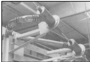
Example of Sonic's Dual Airwipe Heads designed for high-speed throughput.
